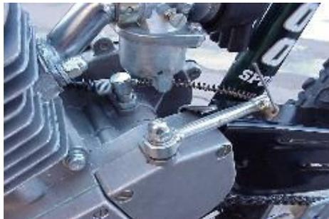
The larger spring is a heat shield for the clutch cable:
