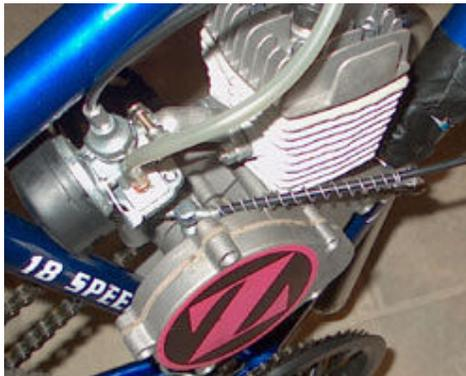
Vibration is a factor with all single cylinder bicycle engines so it is a good idea use a spot of 'Holdtite' or 'Loctite' on all screws and nuts when installing the engine. If the head nuts vibrate loose they will cause the head gasket to blow and if the side cover plates come loose it will let water into the magneto and cause damage to your electrical system. Engine mounts can also vibrate loose.
