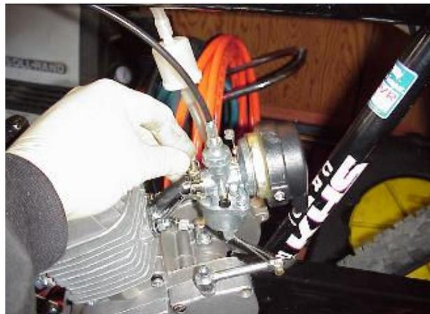
**NOTE:** During run in, keep drive chain snug. During run in keep the mix ratio at 16:1 for 500 kilometers and keep your speed down to a maximum of 20kph and do not run your motor for longer than 30 minute periods.
