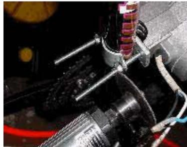
Here is how the front motor mount looks if you have to use the 3 hole adaptor. Yes, you drill and as you can see it works perfectly and you may have to get a longer bolt and bend the exhaust pipe some too. To bend the pipe, simply get a vice and use some wood to block the pipe and then bend it. ZBox has made special galvanised U-bolt adaptor assemblies for \$10 extra if you don't want to drill a hole through your front tube.
