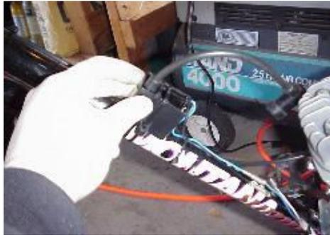
Testing resistance on magneto coil should read:
